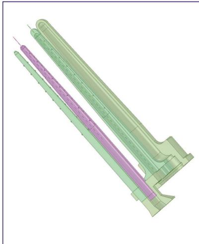
When conducting a flow analysis, the plunger, cooling tube parts, and air volume are created using SpaceClaim.
