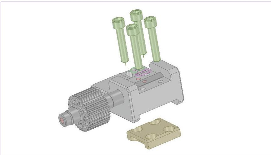
Pusher bracket shows the holding bracket for the pusher that is used to transfer the container to the conveyor belt. SpaceClaim enables the engineering team to simplify the model to include only the metal parts needed for heat transfer analysis.
