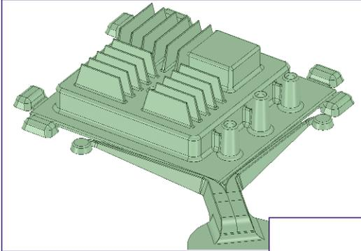
**Figure 2:** The part has been product matured towards the high pressure die casting process. Some holes have been removed and larger radii has been added. This is done in close cooperation with the customer. Using SpaceClaim this has been done in a few hours. In addition a runner and venting system has been applied to the part for the initial CFD analysis.
