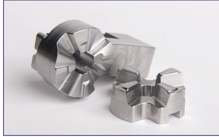
Cam components for 3D surfaces for the automotive industry, milled from solid material. Application area: prototypes for height adjustment of steering column in cars.
