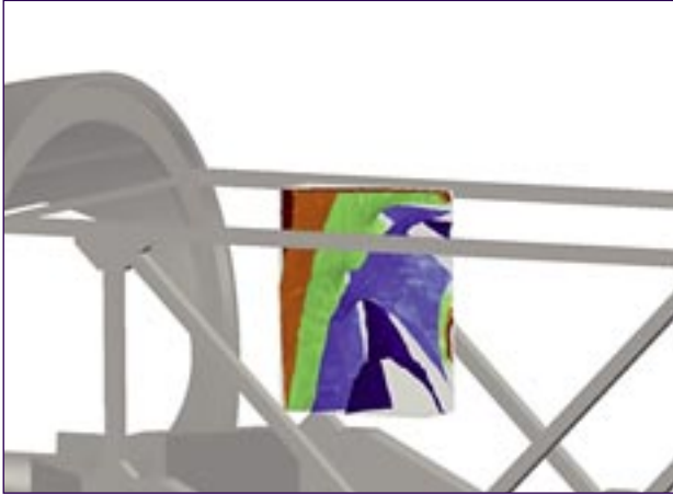
Figure 1: To investigate the magnetic field and determine the requirements for protection at a certain location in the nacelle, a volume of interest is added to the model. The volume could represent a control panel, in which protection might be crucial. The magnetic field is in this case illustrated by an isosurface plot where each color represents different values of the magnetic field.
